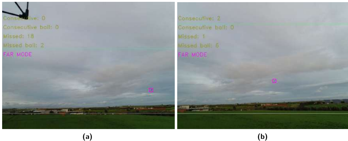
Figure 18. Target UAV detection results from the Long-Range UAV Detector module. The UAV detections are depicted in magenta.
