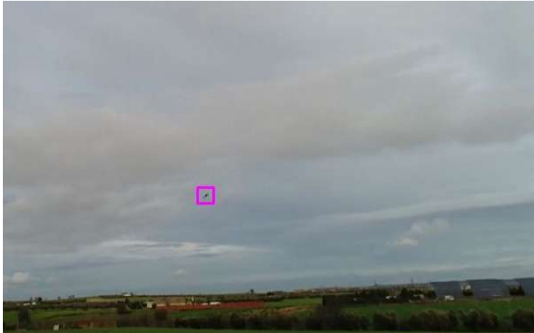
Figure 10. Example of a long-range UAV successful detection. The target UAV appears reduced within the image plane.
