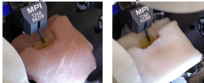
Figure 8: Antenna between human-like tissue measurements. On the left, antenna surrounded by pork muscle tissues. On the right, antenna surrounded by pork fat tissues.
