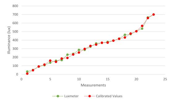
Figure 5. Mobile ambient light sensor vs. Luxmeter.
