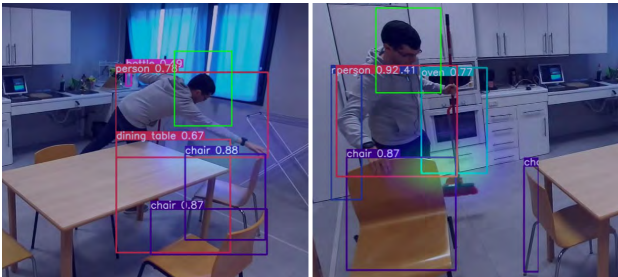
(a) Due to body and object occlusion the output has low confidence (b) The transition frames between actions usually are ambiguous
