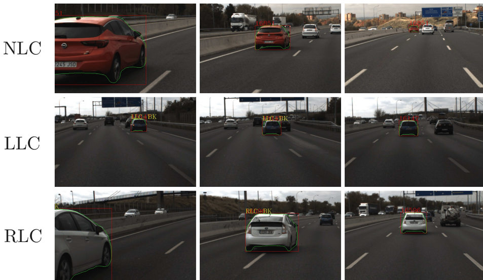
Figure 4.1: Typical sequence representation. No lane-change maneuvers (top) are displayed from beginning to end. lane-change maneuvers (middle and bottom) are represented at the beginning of the maneuver, at the lane change event, and the end of the maneuver.
