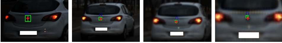
Figure 3.16: Vehicle key point tracking using Median-Flow tracking algorithm. From left to right, tracker initialization and key points after 1, 2, and 3 seconds of tracking. Different zoom levels are applied in each image, 1, 2, 4, and 8 zoom factor respectively.
