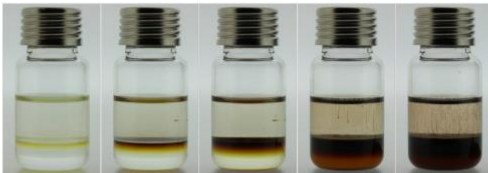
Fig. 1. Pictures of a vial with gasoline 98 RON (upper part) and sulphuric acid (lower part) at 2/3 (v/v) and 1/3 (v/v), respectively. Pictures (from left to right) were taken at 0 h, 3 h, 7 h, 30 h and 48 h after mixing both liquids.
