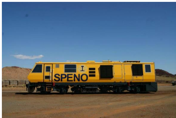
Fig. 1-4 Large-scale track breakage detection vehicle produced by SPENO company
