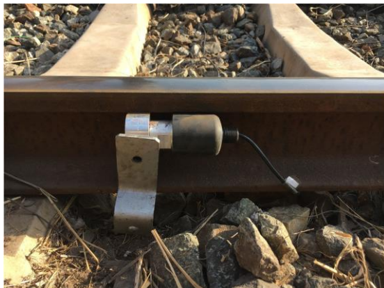
Fig. 4-7 Installation diagram of customized transducer
