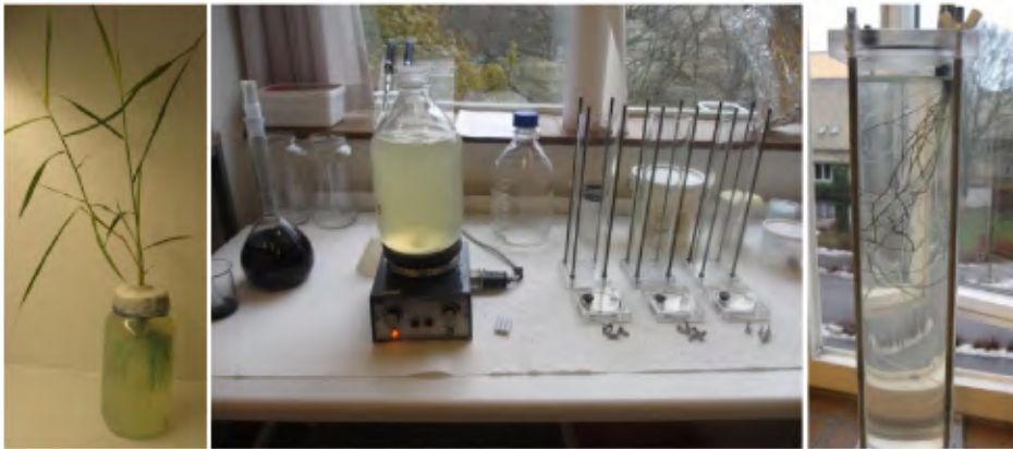
Figure 4-7: Experimental set up of the methylene blue method and examples of plants mounted in two types of jar.
