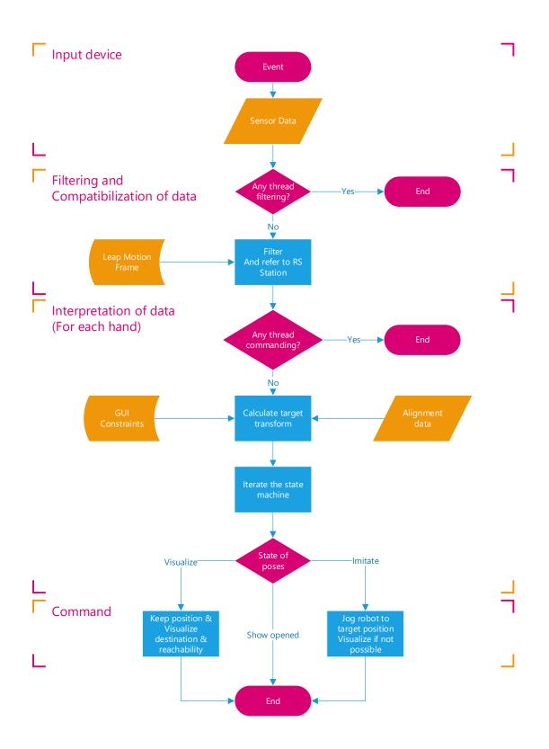
Figure 4.12: Flowchart of the Leap Motion Sensor Input Mode. Interpretation stage is done for each hand, with different state machines. Feedback sent to the GUI is excluded in this representation.
