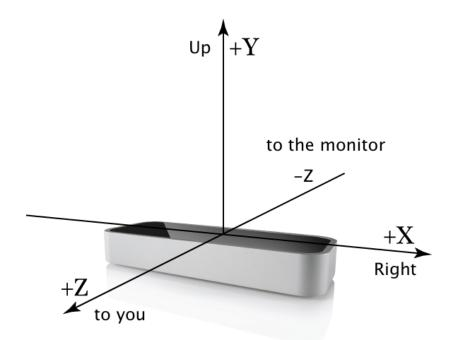
Figure 4.11: Leap Motion Sensor axes. Values given by the sensor are referred to these axes.
