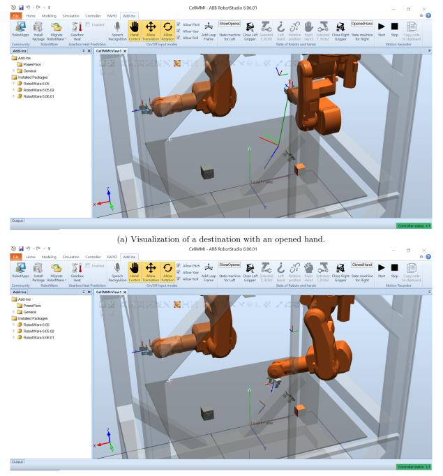
(b) Robot moved to a destination with closed hand, the robot moves as long as the hand is closed.
