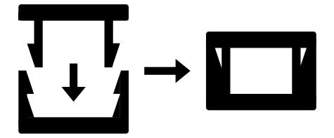
Figure 3.2: Snap-fit insertion.
