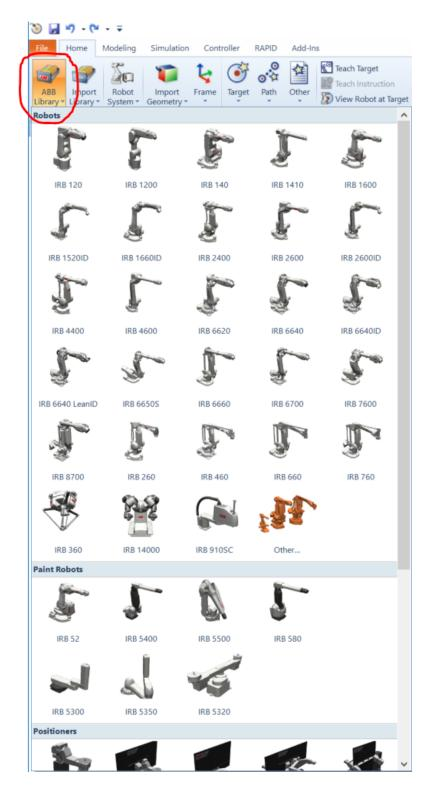
Figure 4.4: How to add robots to the station, using the RS GUI and their library.
