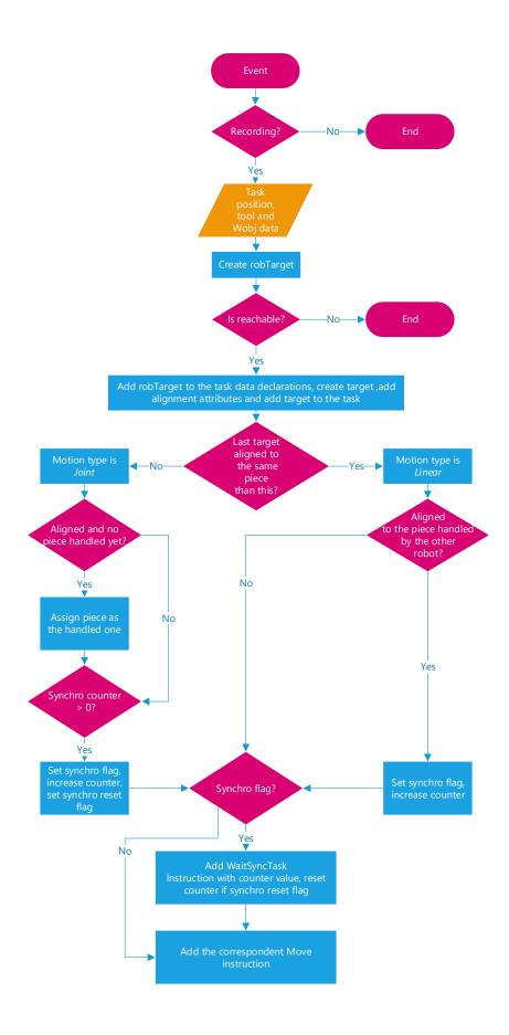
Figure 4.17: Flowchart of the target recording. Flags are reset on every order.
