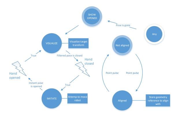
Figure 4.13: State machine for each hand. Lightning symbols represent triggered events.
