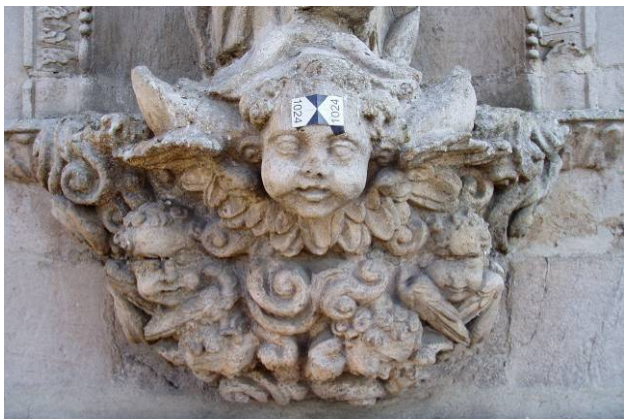
Fig. 5. Type of targets used for control points
