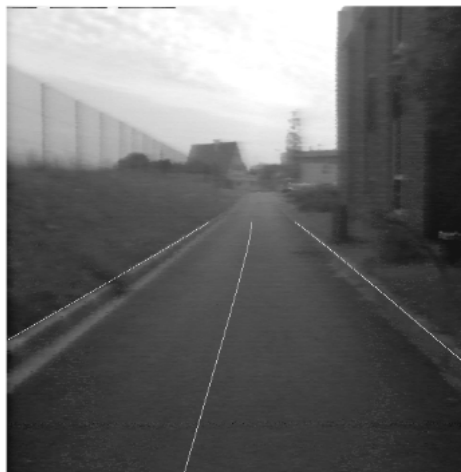
Figure 2.11: Image with bad contrast but well marked lane boundaries using splines
