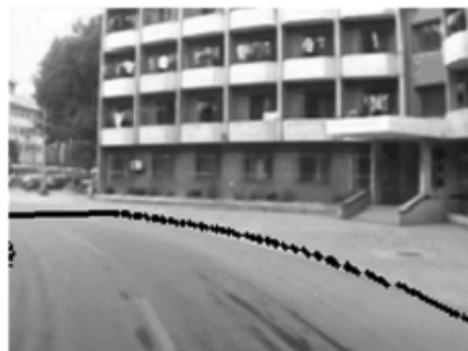
Figure 2.8: Result of road detection in a curved roads in color-based road segmentation [20].
