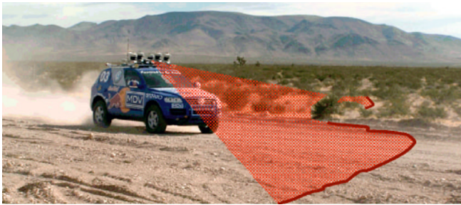
(a) Illustration of a laser sensor: The sensor is angled downward to scan the terrain in front of the vehicle as it moves. Stanley possesses five such sensors, mounted at five different angles.
