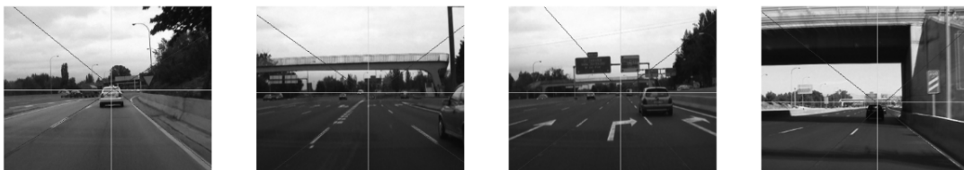
Figure 2.16: Several examples of vanishing point estimation and road model extraction. Example (a) shows the most simple case where the road is almost empty, while cases (b) and (c) are quite more difficult as there are overtaking traffic and road traffic signals that difficult the correct detection. Case (d) shows a particular situation where the illumination conditions have abruptly changed due to the shadow casted by a bridge on the road.
