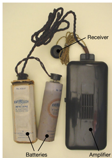
Figure 2.8: A relatively late vacuum tube hearing aid. The microphone, amplifier and the two batteries were combined into a single body-worn electrical hearing aid, which connected to a receiver placed in the ear by means of a wire.
