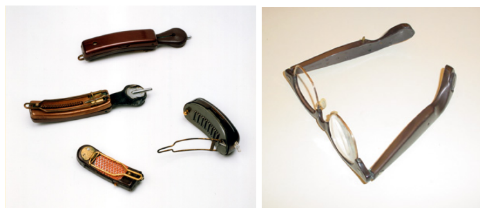
Figure 2.10: First analog hearing aids worn completely in the head. In (a), it is shown several barrette hearing aids, which had an external receiver like a body aid, and in (b), it is depicted an eyeglass aid, in which all the components were included into the device.
