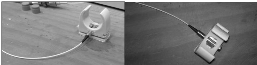
Figure 2. The modified Faraday mirror, packed with the additional neodymium magnets and a holder, ready to be directly adapted to the railway catenary.
